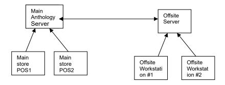
Fig 1- Typical Offsite setup, Offsite Sever laptop can run Main Anthology and Offsite copy with 2 other laptops that can only run the Offsite copy from the Offsite Server.
